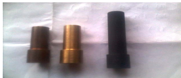
Fig. 1: Shows brass,copper graphite electrode(dia 15mm)
